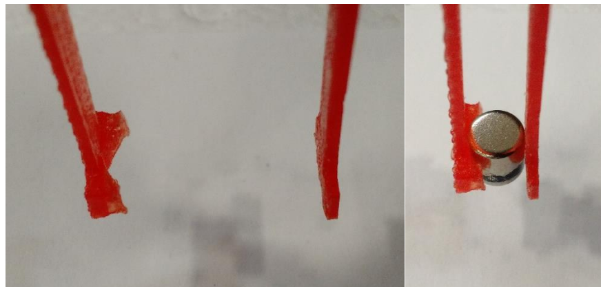
Figure 4-5: Fingertip design 2. The shallow “V” shape on the left fingertip causes the gripper to self-center cups as it grasps them. Left: gripper open. Right: grasping a cup.
