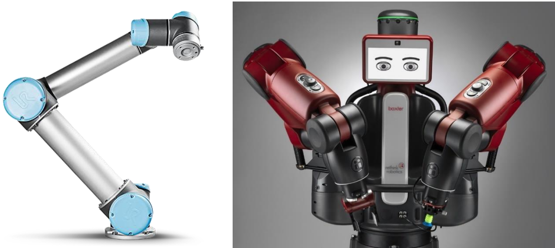
Figure 1-1: Examples of the two types of robot on the market today. Left: Universal Robots UR5, a 6-degree of freedom industrial manipulator [8]. Right: Baxter, a dual-arm collaborative robot platform that uses series elastic actuators [7].
