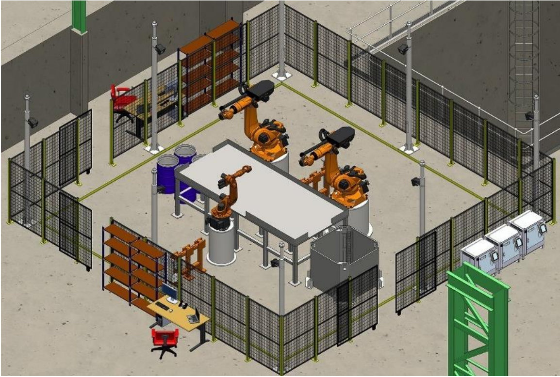
Figure 1-3: The RoMaNS segregation and sorting system testbed [14].
