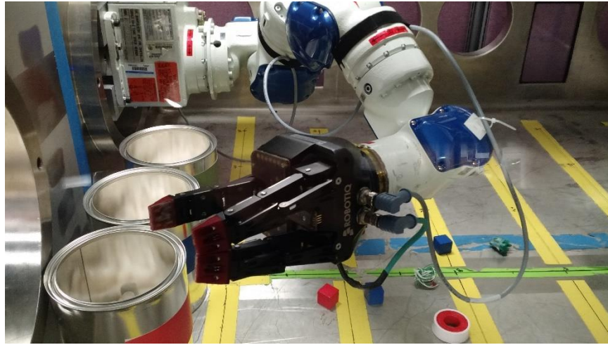
Figure 6-4: The robot shortly after sorting an object into a waste container (pseudocode line 10). This picture was taken from the approximate viewpoint of the RGBD camera mounted on the glovebox.
