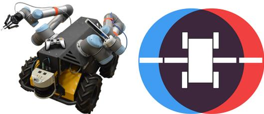
Fig. 2: The VaultBot dual-arm mobile platform (left). Schematic showing the VaultBot’s workspace for each manipulator (right UR5: blue, left UR5: red), viewed from above (right). Figure best viewed in color.
