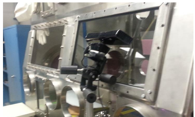
Fig. 8. Glovebox with camera outside glovebox window
