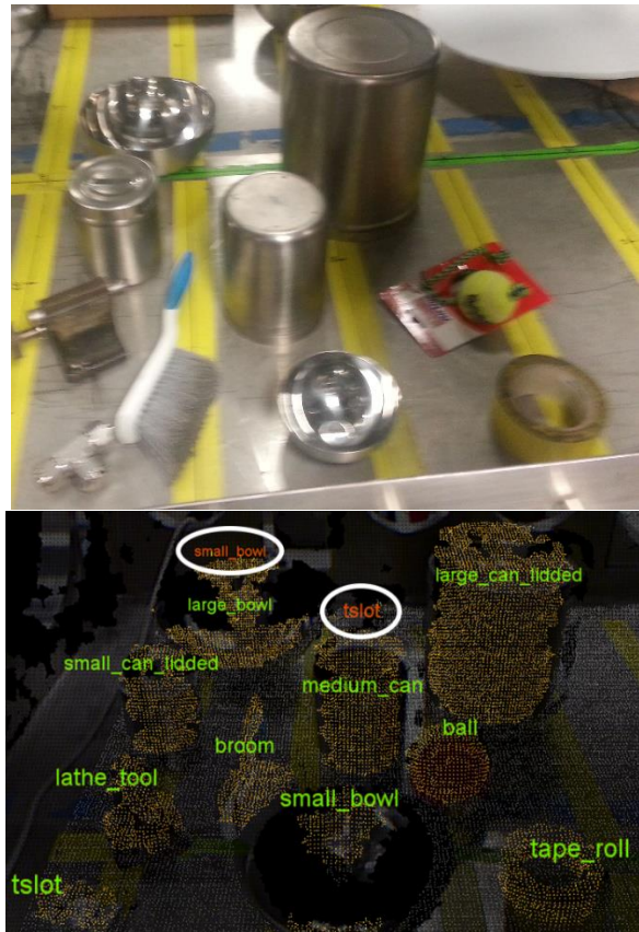
Fig. 7. Cluttered scene with recognition results and a reproduction of the scene in the glovebox
